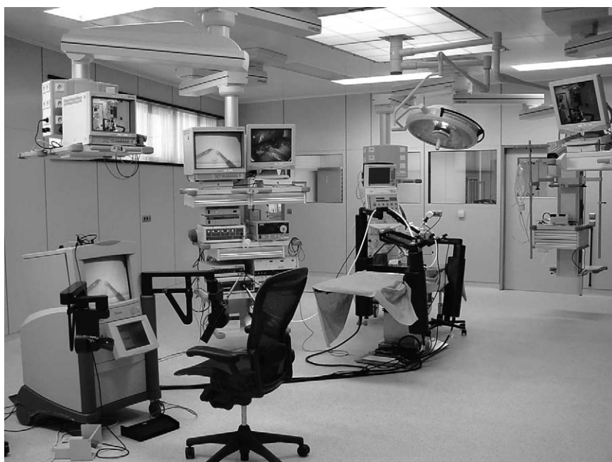
Fig. 1. The ZEUS subsystems: the surgeon’s robotic console; robotic arms on the patient’s side.
